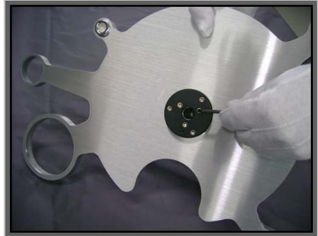
Assembling the spindle holder to the sub-chassis
