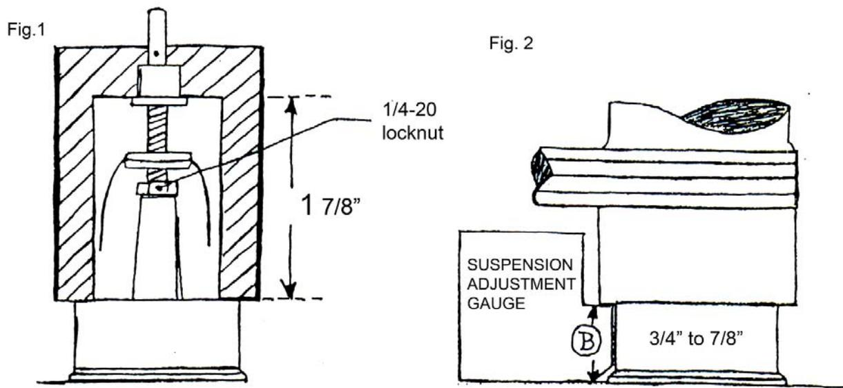
note : The gauge shown in fig. 1 can be made with cardboard.
