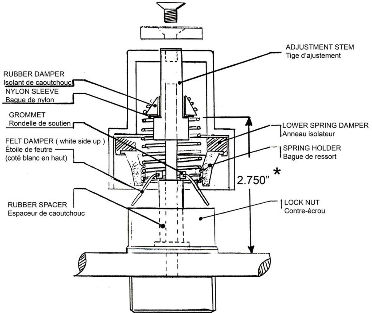
\* Adjust the height of the adjustment stem at 2.750" ( 69.85mm ) as the first procedure to calibrate the suspension.
