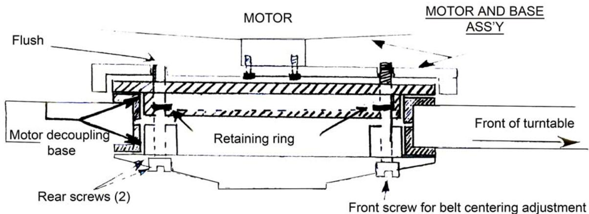
NOTE: If those screws are turned in too far, not enough motor angle adjustment will be provided. The front screw will be used for the fine adjustment of the belt tracking in the pulley of the motor. This adjustment should only be done once the acrylic base and subchassis are properly leveled.
