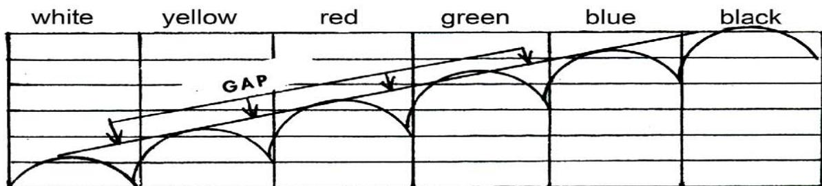
We re-evaluated the different suspension loads to be covered to accommodate all the tone arms that can be mounted on the Oracle. We came out with the following color coded springs, from the weakest to the strongest, white, yellow, red, green, blue, black (almost never used was required for the very heavy tone arms). The major difference is the spring support, which makes it possible to almost eliminate the gap between each spring as shown on graph II.
