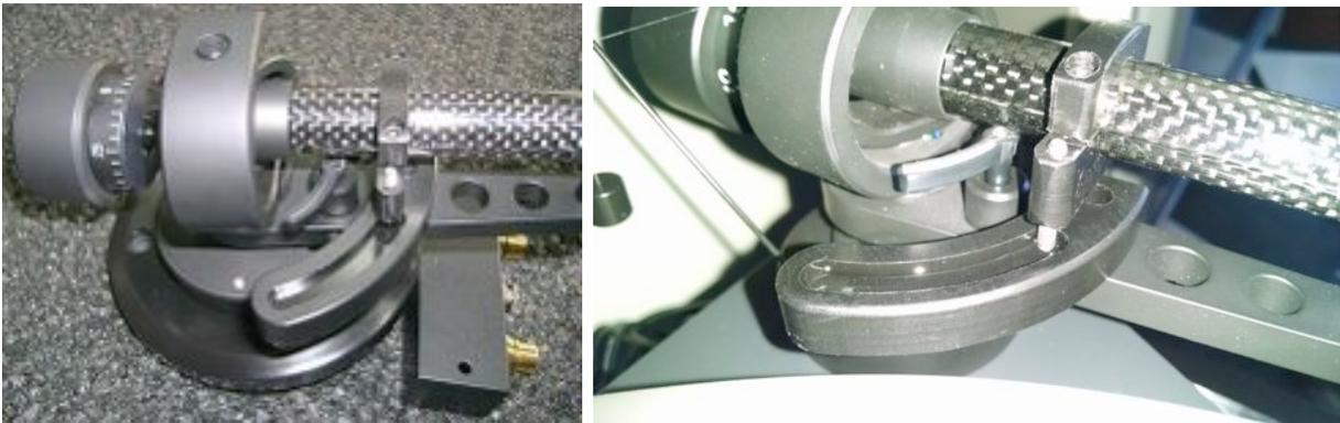
1. **After removing the anti-skating weight**, set a flat record on the platter - set the stylus on the record.
